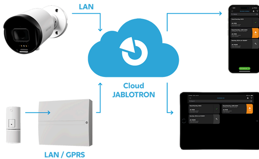
Fig. 2: Diagram of JABLOTRON CLOUD functioning
