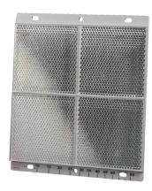
The Opal addressable beam detector is an intelligent reflector type linear optical beam smoke detector designed to operate with Notifier addressable fire alarm systems. It operates primarily on the principle of light obscuration utilising infra-red light.
